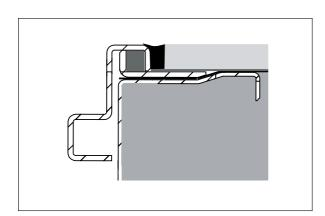
Make sure the clamping frame holds the sealing membrane securely.
