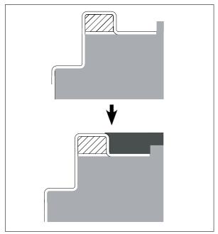
Lay out a strip in order to make a recess in the concrete, see illustration
