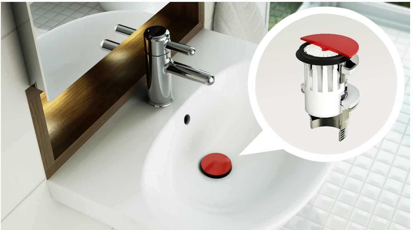
PUM - Purus Universal Membrane, is a revolutionary membrane which stops bad air to come up through the drainage system. The new technique saves space without reducing the flow capacity and is also functioning as an air admittance valve when there is a negative pressure in the drainage system (secondary air ventilation). This gives much better flow in the drainage pipe. PUM works also to a certain extent as a back flow stop.
